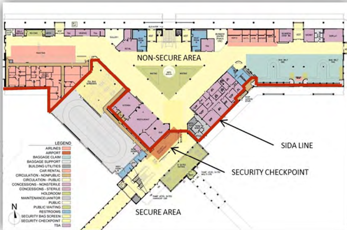
The existing non-secure area, showing the Security Identification Display Area, (SIDA), line
