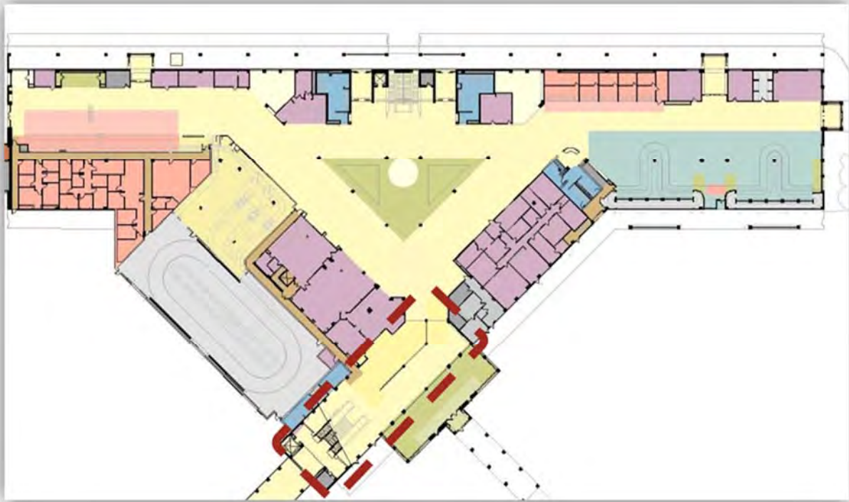
The existing security checkpoint and vertical circulation areas
