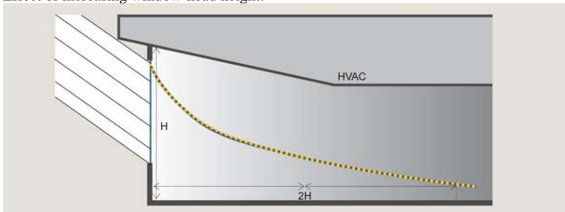
Effect of placement of light shelving at exterior (exterior/interior shelf provides the more even light distribution, but not necessarily the deepest):
