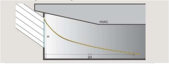
Effect of placement of light shelving at exterior (exterior/interior shelf provides the more even light distribution, but not necessarily the deepest):
