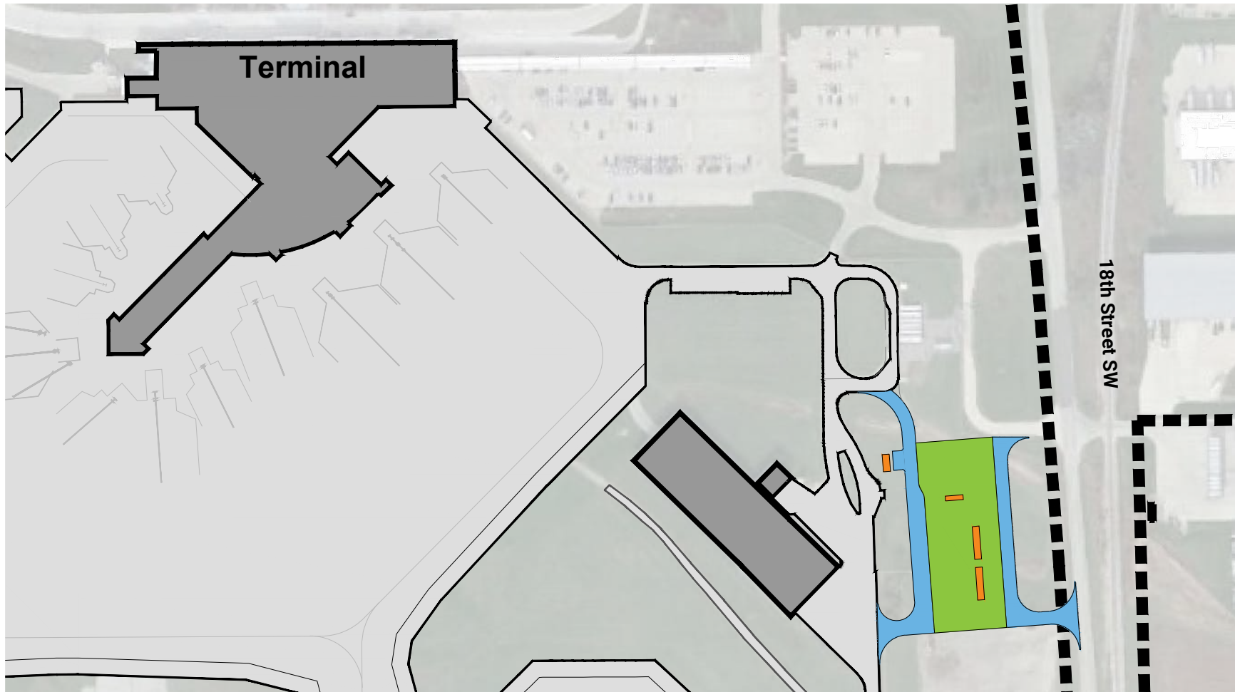
Figure 4.11: Fuel Farm Location
